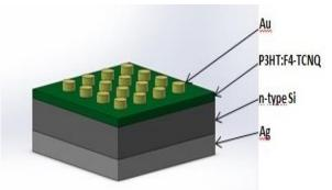
Figure 1.Au/P3HT:F4-TCNQ/n-Si diode structure.
