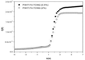
Figure 4.The F4-TCNQ concentration dependent capacitance-voltage characteristic for Au/P3HT:F4-TCNQ/n-Si MPS SBDs at 1MHz.
