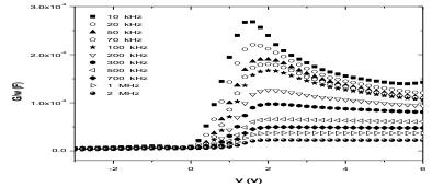
**Figure 8.**The frequency dependent conductance-voltage characteristic of 2% F4-TCNQ used Au/P3HT:F4-TCNQ/n-Si SBD.
