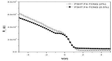
Figure 5.The frequency dependent R<sub>i</sub>-V characteristic comparison of 0.5% and 2% F4-TCNQ concentration used Au/P3HT:F4-TCNQ/n-Si SBDs at 1MHz.
