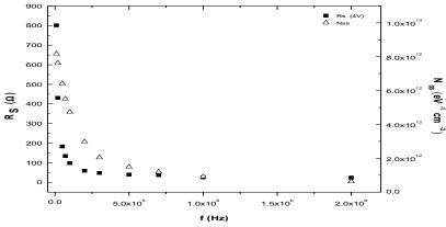
Figure 12. The variation of N<sub>ss</sub> and R<sub>s</sub> for various frequencies for the Au/P3HT:F4-TCNQ/n-Si Schottky barrier diode
