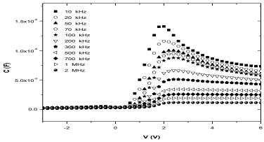
Figure 7.The frequency dependent capacitance-voltage characteristic of 2% F4-TCNQ used Au/P3HT:F4-TCNQ/n-Si SBD.
