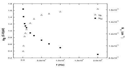
**Figure 11.**The\u03c6<sub>B</sub>(C-V)and N<sub>D</sub> parameters for various frequencies for the Au/P3HT:F4-TCNQ/n-Si Schottky barrier diode
