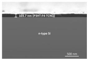
Figure 3. Cross-sectional SEM image of P3HT:F4-TCNQ/n-Si structure with 2% F4-TCNQ concentration.
