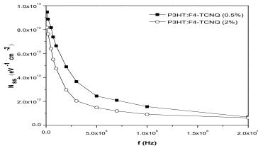
Figure 6.The frequency dependent N<sub>ss</sub> characteristic for 2% and 0.5% F4-TCNQ concentration used Au/P3HT:F4-TCNQ/n-Si MPS SBDs.
