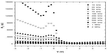
Figure 9.The characteristics of diode resistance (R<sub>i</sub>) for various frequencies of the Au/P3HT:F4-TCNQ/n-Si Schottky barrier diode at room temperature.
