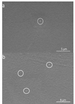
Figure 2.SEM images of (a) 0.5% F4-TCNQ and (b) 2% F4-TCNQ concentration used P3HT:F4-TCNQ surfaces.
