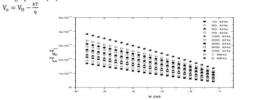
**Figure 10.**The C<sup>-2</sup>-V plots of the Au/P3HT:F4-TCNQ/n-Si Schottky barrier diode at room temperature as a function of voltage
