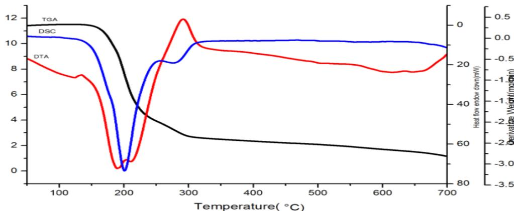
**Fig 7:** TG/DTA/DSC curves of pure and doped BTZA
