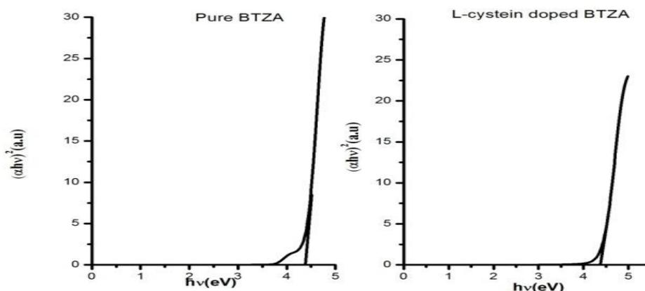
**Fig 5:**  $(\alpha hv)^2$  versus photon energy ( $h\nu$ ) of pure and doped BTZA
