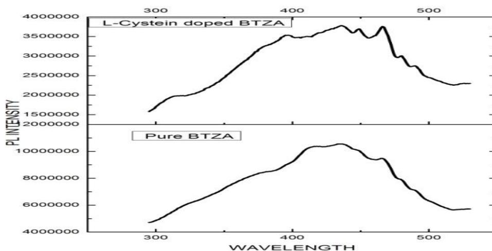
**Fig 6:** Photoluminescence spectrum of pure and doped BTZA
