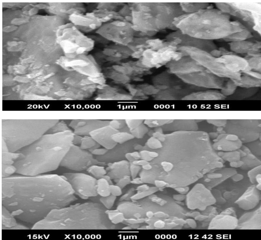
**Fig 3:** SEM images of Pure and doped BTZA crystal
