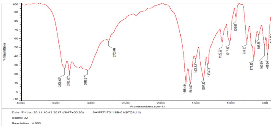
**Fig 8:**FT-IR spectrum of doped BTZA crystal
