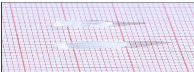
Fig 1: Photograph of L- BTZA single crystal
