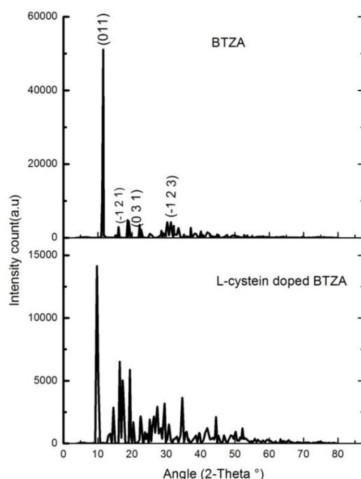
**Fig 2:** Powder XRD pattern of pure and doped BTZA
