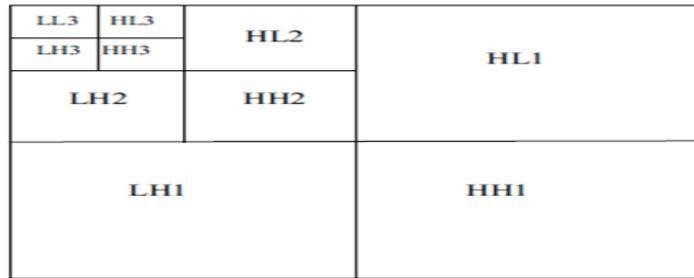
Fig.4.3 3 level discrete wavelet transform
