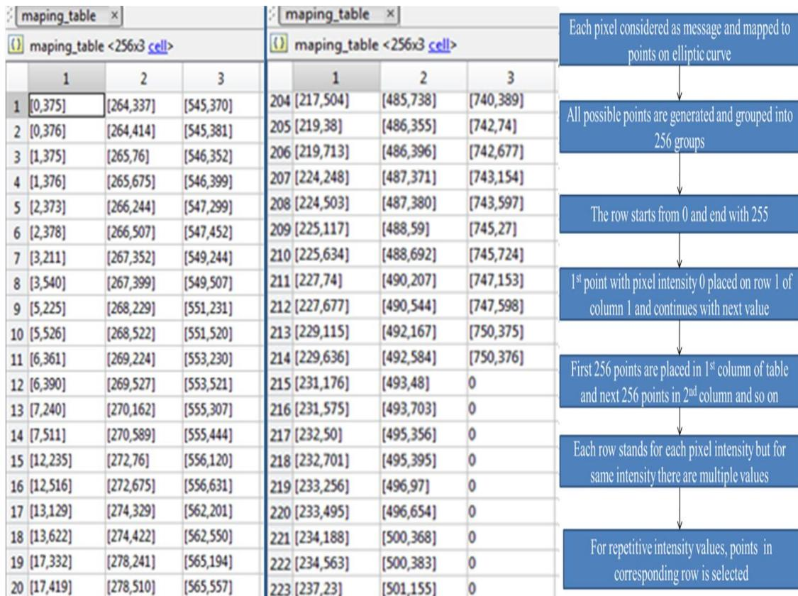
Fig.4.2points generated by using the mapping methodology
