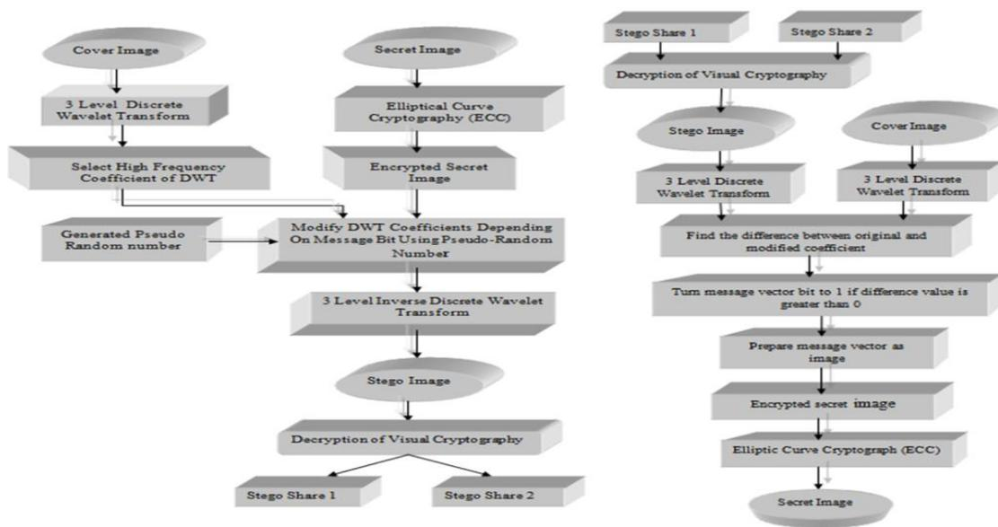
Fig 3.1. Block diagram of proposed method, Sender end and Receiver end
