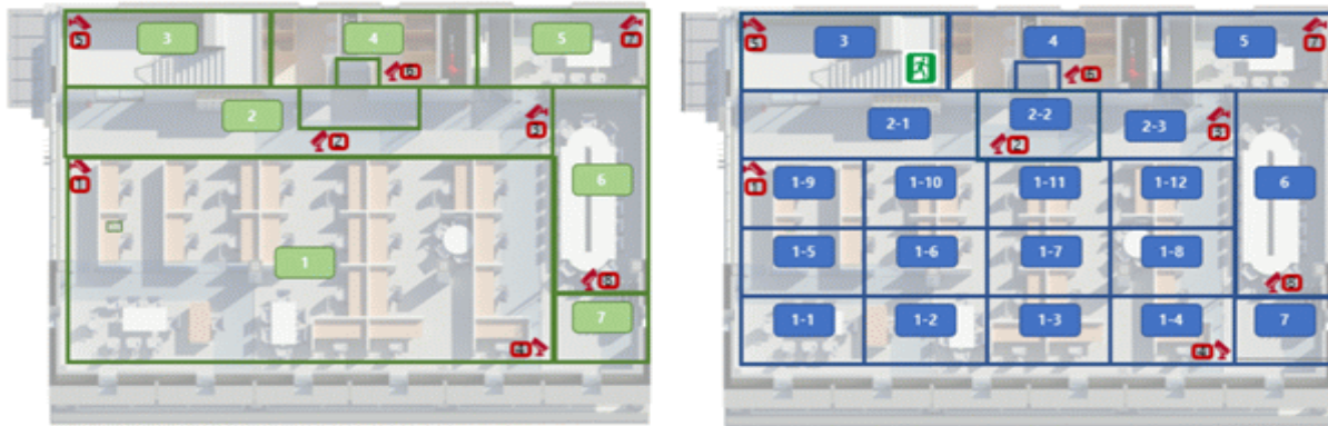
Fig. 3. Fire partition and CCTV position (Left) / Space partition for transmission monitoring (Right)
