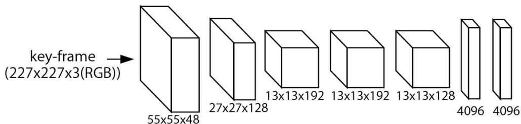
Fig 2: Architecture of Deep CNN [5]
