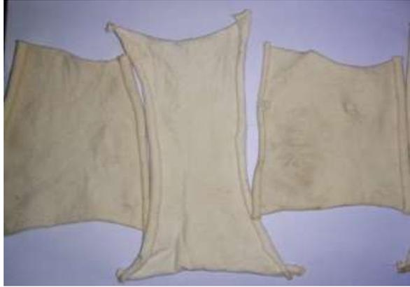
Figure 2: Sample after normal water wash ability test
