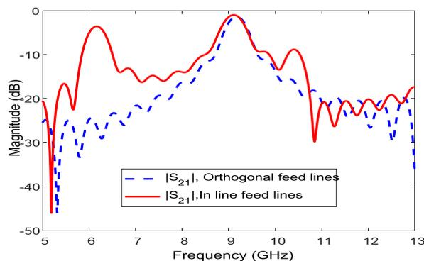
**Figure 3.** Insertion loss of octagonal ring resonator for different port's location.
