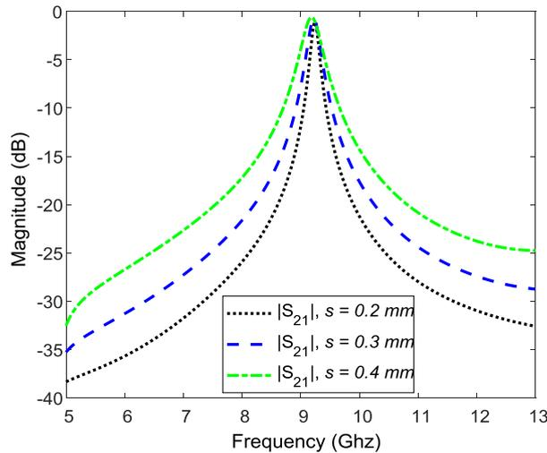
Figure 4. Insertion loss of the proposed filter for different gap values.
