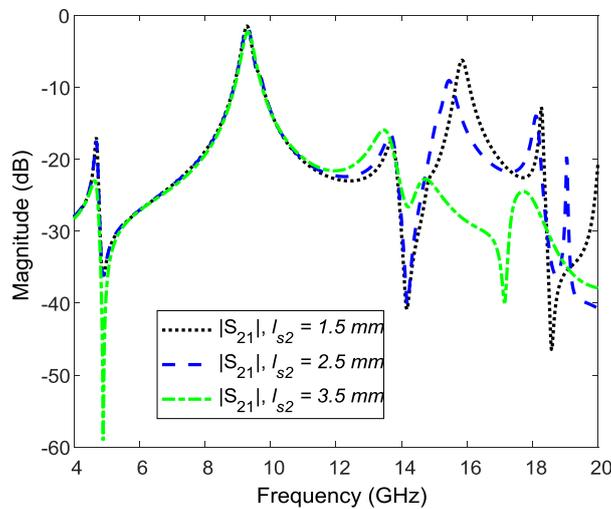
Figure 5. Insertion loss of the proposed filter for different DGs length.
