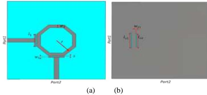
**Figure 1.** (a) Top view and (b) bottom view of the proposed narrowband passband filter.
