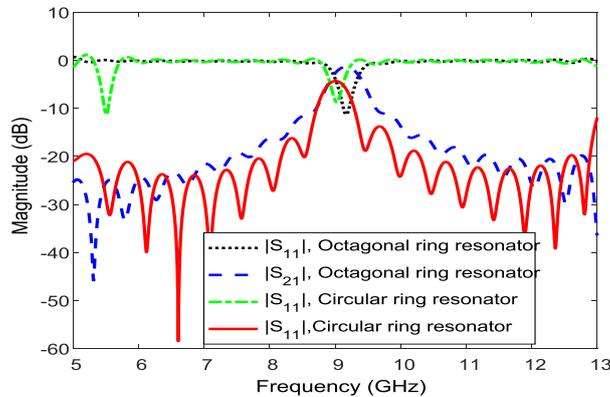
**Figure 2.** S-parameters of octagonal and circular ring resonators with same radius.
