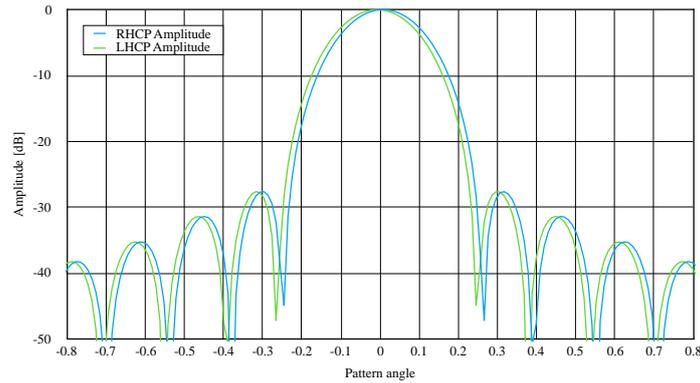
**Fig. 2.** Normalized pattern of the offset-parabolic-reflector antenna with circularly polarized feed.
