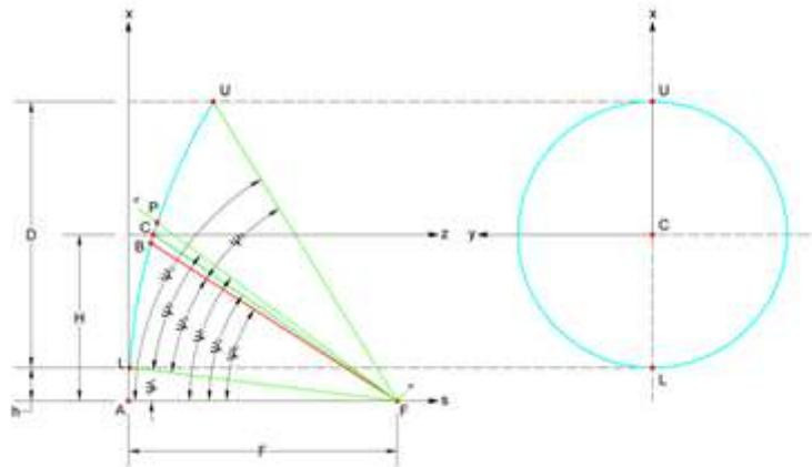
Fig. 1. The geometry for the offset-parabolic-reflector antenna, [1].
