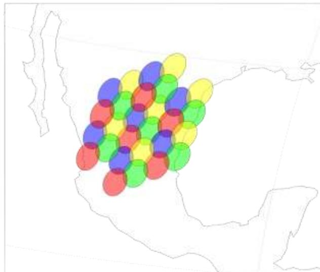
**Fig. 4.** Four-cell reuse scheme for a four-reflector design in Ka band for a beamwidth = 0.32°.
