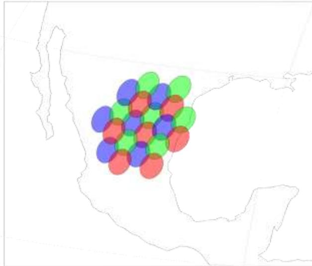
**Fig. 3.** Three-cell reuse scheme for a three-reflector design in Ka band for a beamwidth = 0.32°.
