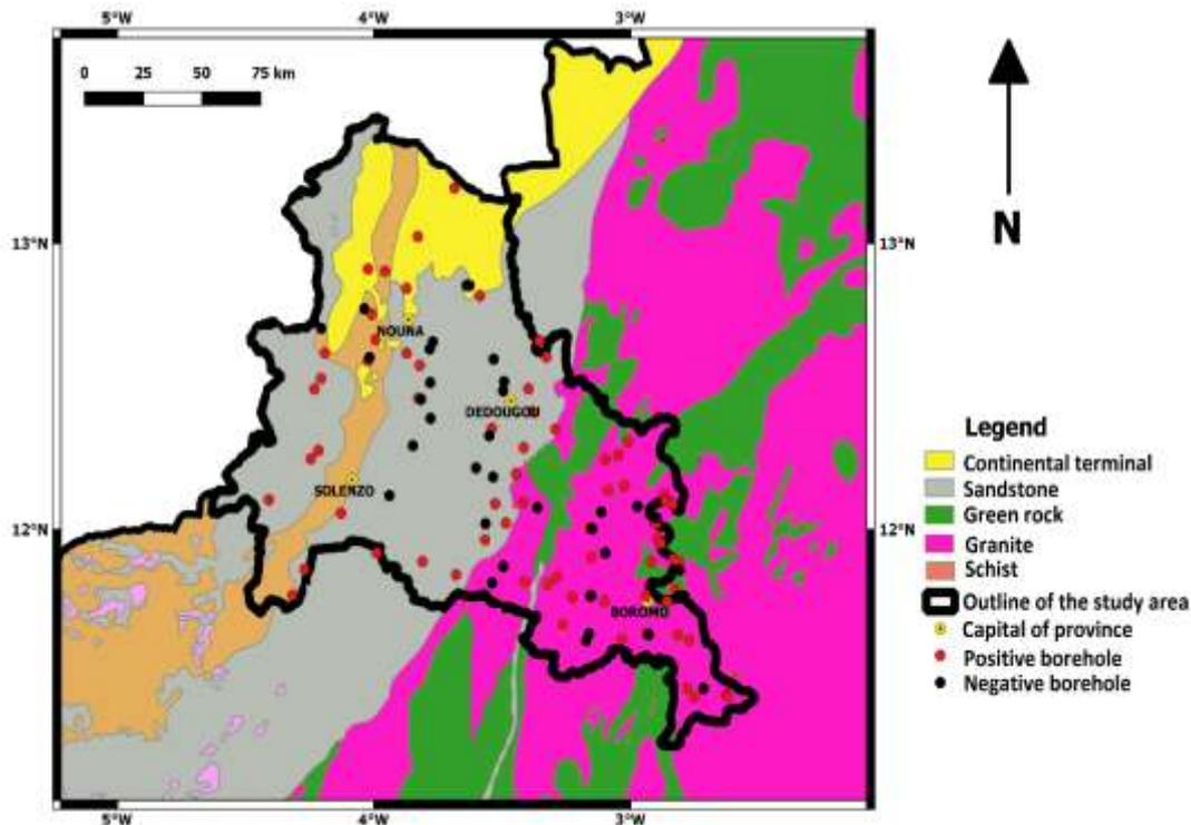
**Figure 2:** Location of the different boreholes
