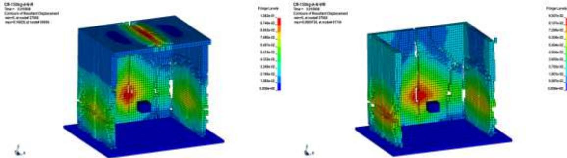
**Figure (14)** Room with and without roof 150kg TNT- Debris Scatter & Displacement at Time = 0.01sec.
