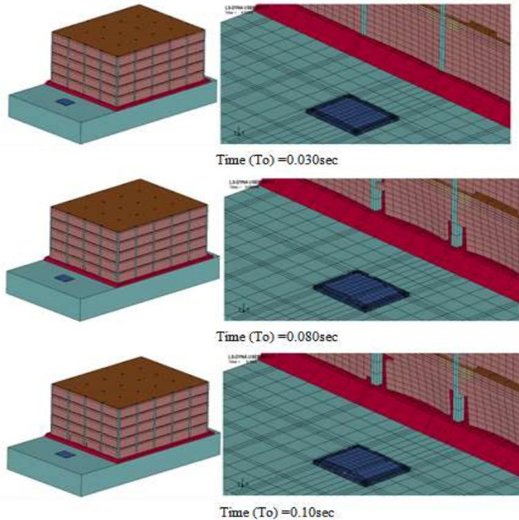
**Figure(27)** Series of images showing the failure and debris scatter of Closed Room and the Factory main elevation concrete walls and columns.
