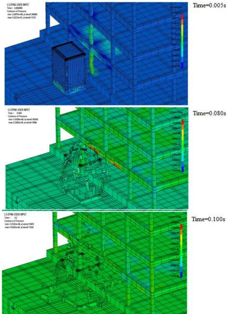
**Figure(24)** Series of images showing the pressure and the damage of the Boiler Room and the Factory main elevation concrete walls and columns.
