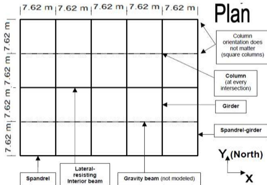
(A) Reinforced Concrete Factory Plan
