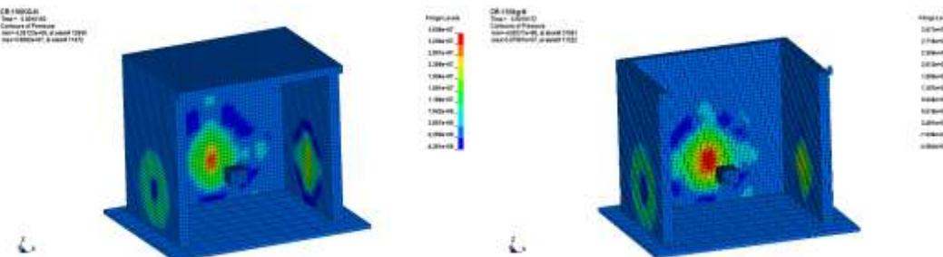
Figure (11) Room with and without roof 150kg TNT-Pressure at time = 0.001sec.
