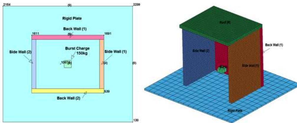
**Figure(3):**3D Model of boiler room –Plan&Perspective View.
