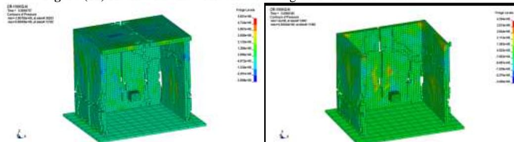
Figure (12) Room with and without roof 150kg TNT-Pressure at time state T0= 0.0066sec.
