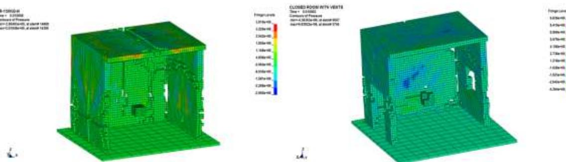
Figure(19) Room with and without Vents 150kg TNT–Pressure at time = 0.01sec.
