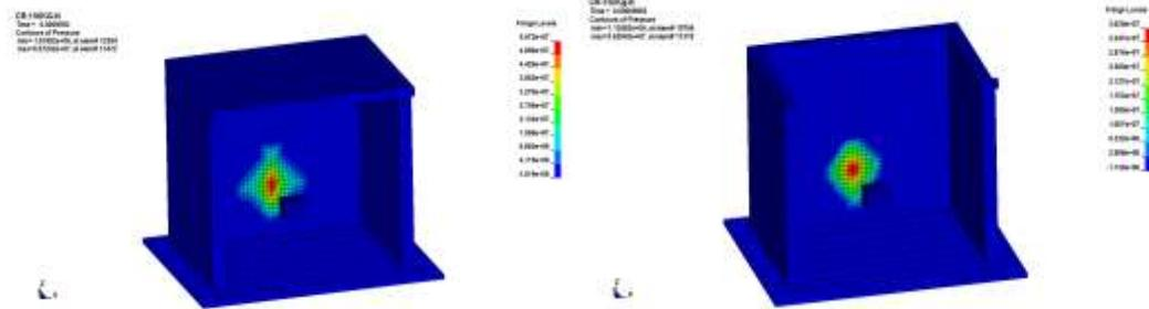
Figure (10) Room with and without roof - 150kg TNT-Pressure at time = 0.0006sec.
