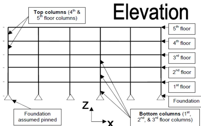
(B) Reinforced Concrete Factory Elevation
