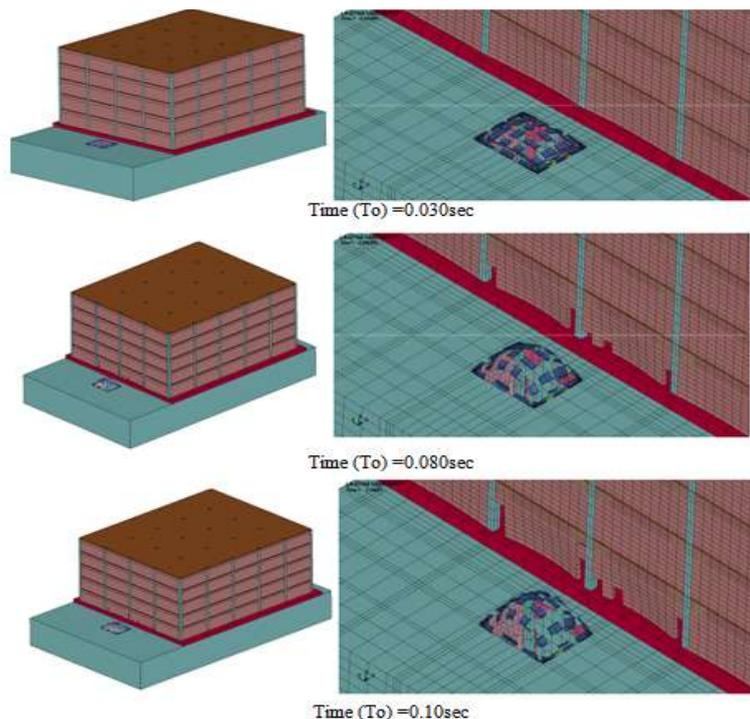
**Figure(26)** Series of images showing the failure and debris scatter of Closed Room and the Factory main elevation concrete walls and columns.
