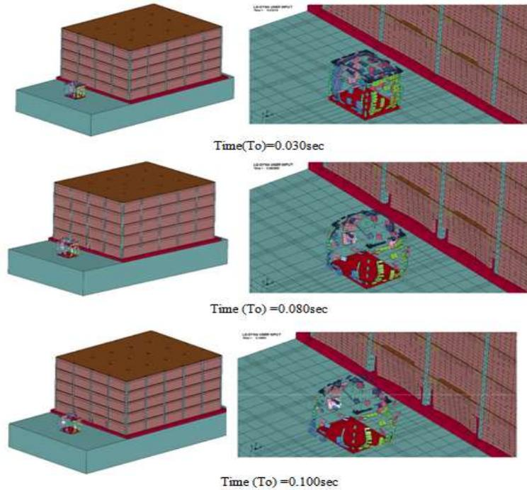
**Figure(25)** Series of images showing the failure and debris scatter of Closed Room and the Factory main elevation concrete walls and columns.
