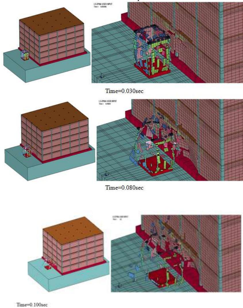
**Figure(23)** Series of images showing the failure and debris scatter of Closed Boiler Room and the
