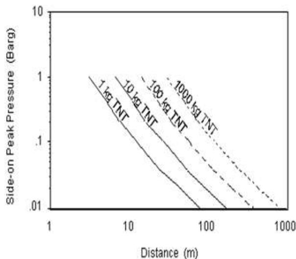
**Figure(2):** Peak explosion pressure (side-on) vs. distance for TNT groundburst. [Gas Explosion Handbook (2007)]
