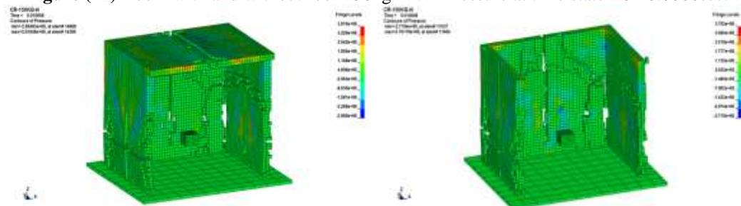
Figure (13) Room with and without roof 150kg TNT-Pressure at time = 0.01sec.
