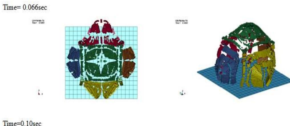
**Figure (8):** Series of images showing the failure and debris scatter of Closed Room -150Kg TNT Equivalent charge.
