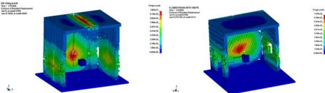
Figure(20) Room with and without Vents 150kg TNT- Debris Scatter & Displacement at Time = 0.01sec.
