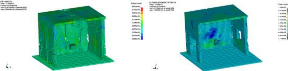
Figure(18) Room with and without Vents 150kg TNT–Pressure at time = 0.0066sec.
