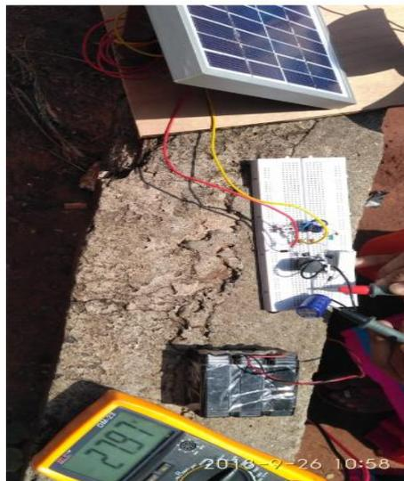
**Figure 17(b).** Output of boost converter circuit when the input was given by solar panel
