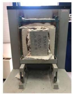
Figure 1 : Set up of fire test
