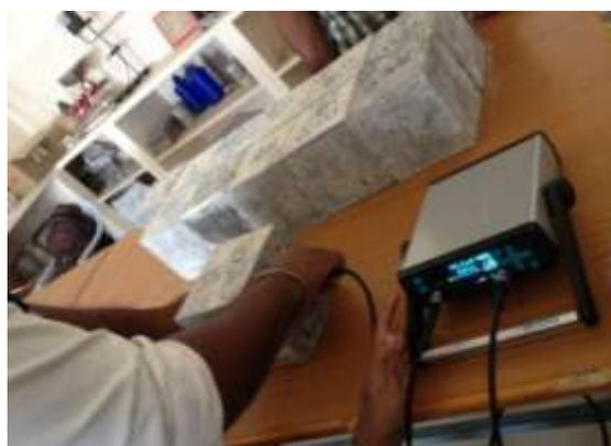
**Fig.3.2 Ultrasonic Pulse Velocity test of cubes**
