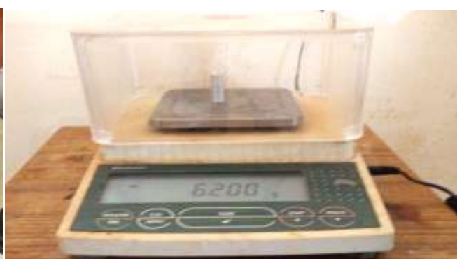
Fig.: weighing of aluminum alloy specimens
