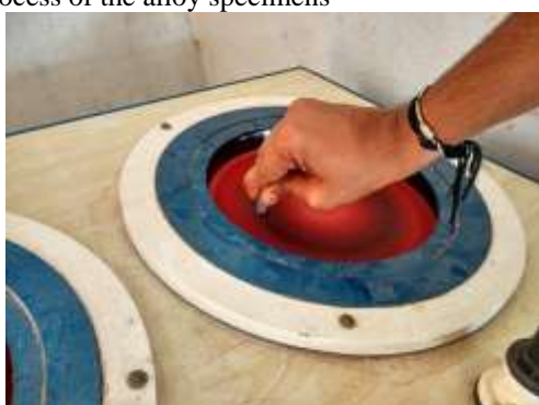
Fig.: Surface finishing of Aluminum alloy Specimens
