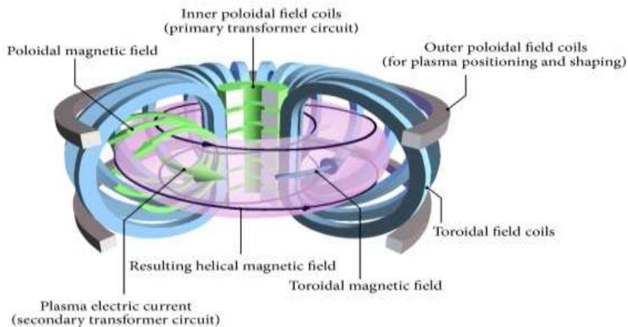
**Fig 2. Tokamak representation**
