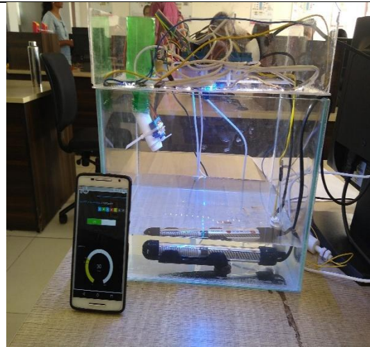
Fig 2. Lighting control through Adafruit IO dashboard
