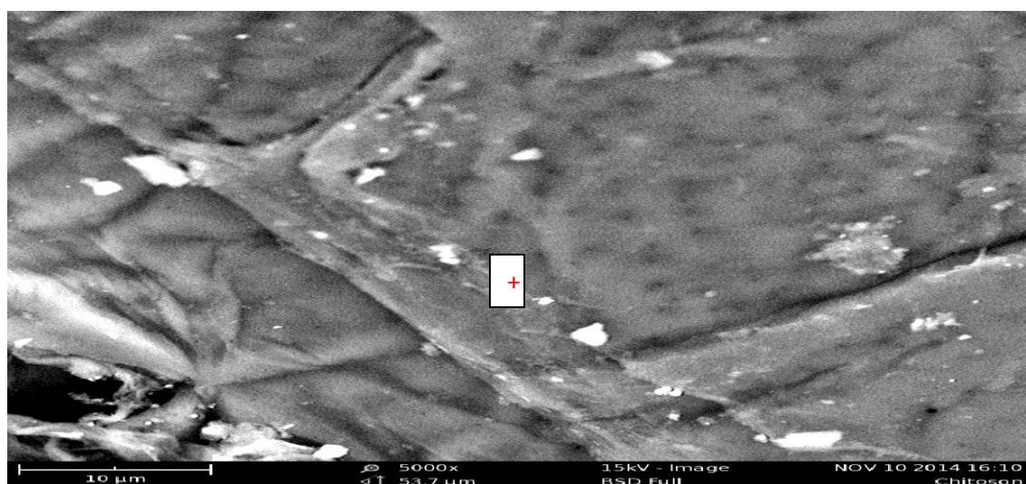
Plate 1: SEM image of Chitosan
