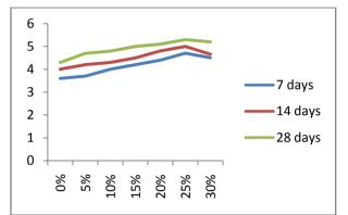
Fig No.4.5 Impact of Granite Powder on Flexural strength of Matrix
