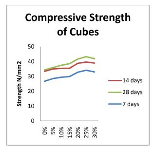
Fig No.4.1 Impact of Granite Powder on Compressive Strength of Matrix
