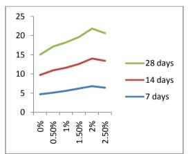
Fig No.4.6 Impact of Steel Fibers on Flexural strength of Matrix
