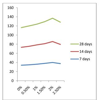
Fig No.4.2 Impact of Steel Fibers on Compressive Strength of Matrix
