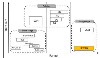
Figure 1. The amount of data and the distance of wireless communications technologies [2]
