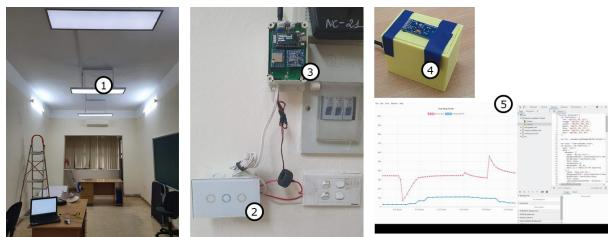
1 – 3 smart LED lights; 2 – Control panel; 3 – Electronic WiFi-integrated power meter; 4 – WiFi-integrated illuminance sensor; 5 – Real-time graph of power and illuminance by time
