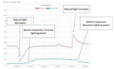
Figure 6. Real-time graph showing the change in power consumption and the stability of illuminance on the desk when the external light is changing
