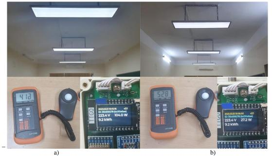
a) External light is ON: power consumption is 104W, illuminance is 418 lux; b) External light is OFF: power consumption is 27W, illuminance is 528W
