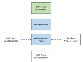
Figure 2. Diagram of an UDP sensor network for short range experiments
