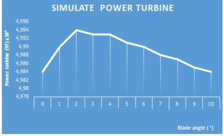
Fig. 5. Simulation values for the generated power of the turbine at v = 5 m/s
